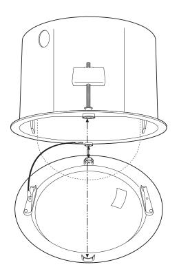
Figure 15. Lower Dome Installation, In-Ceiling Models
